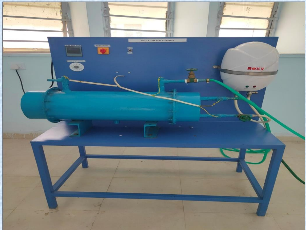
Shell and tube Heat exchanger Apparatus
